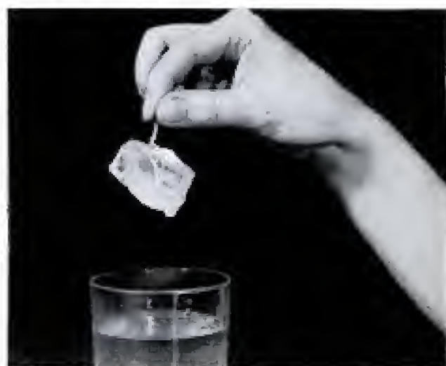
Using just a paper match, lift the ice cube from the water. This one is a real fooler. Drop a pinch of table salt on the ice and hold the match against it. Ice melts and refreezes to "cement" match to cube
